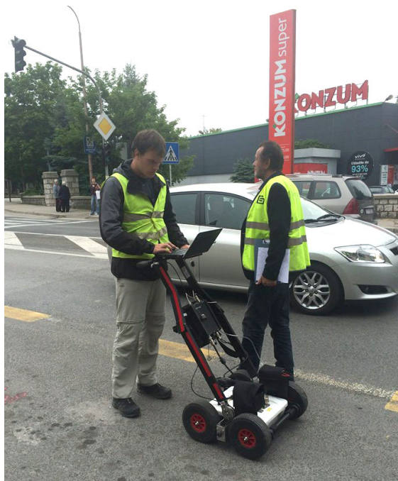
Figure 2: Employees of Geoprojekt d.d. during field work with a ground penetrating radar
