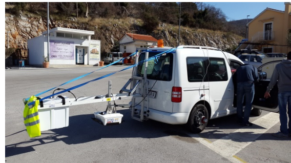
Figure 3: Vehicle-mounted double-antenna Hi-Pave system
